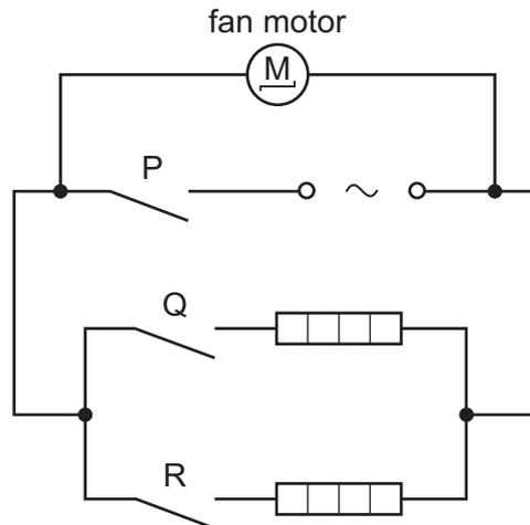
The fan motor has a power rating of 0.10 kW and the heaters each have a rating of 0.40 kW. The cost of electricity is 8.0 cents / kWh.
