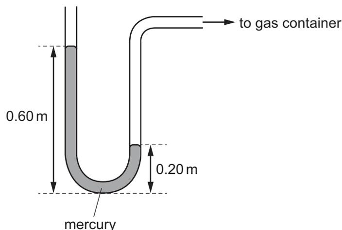
The density of mercury is  $14\,000\text{ kg/m}^3$ . The gravitational field strength  $g$  is  $10\text{ N/kg}$ .
